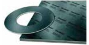
High performance graphite material with multiple plain stainless steel foil inserts bound by a proprietary technology without using adhesives. MLX is suitable in heavy-duty conditions because of its very high compressive strength. An excellent choice for high pressure applications. MLX gaskets are robust and adapt to any sealing surface including irregular flanges. Chose from 1, 2, 3, 5 or 7 layers of 316(L) reinforcement inserts.
