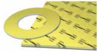
A special multi-layer gasket material with improved flexibility at higher temperatures. This material is resistant to creep and cold flow. KLINGERSIL® top-sil ML1 is manufactured with a revolutionary combination of synthetic fibers and HNBR and NBR rubbers, reinforced in a multi-layer structure. This unique multi-layer structure extends service life.
