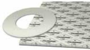
Gasket material is specifically designed for an aggressive chemical environment. It is resistant to most mineral acids and alkalis, ketones, and aldehydes. C-8200 is manufactured with a unique blend of glass fibers reinforced with a special acid-resistant binder.
