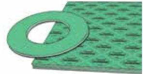
A universal material that is resistant to oils, water, steam, gases, salt solutions, fuels, alcohols, moderate organic and inorganic acids, hydrocarbons, lubricants, and refrigerants. C-4400 is manufactured with aramid fiber reinforced with a nitrile binder.
