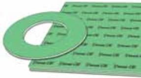
A general service compressed non-asbestos gasket material with a wide range of application potential. Use it in general applications. 400 MAX is manufactured with quality fibers, fillers with a nitrile binder (NBR). This material has a temperature range of -40°F to 400°F.
