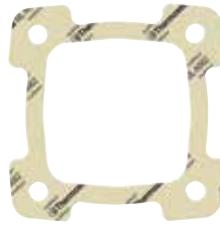
ML-N562 is synthetic fiber and nitrile butadiene gasket material designed for difficult sealing applications with very low flange pressure or very rough surface finishes. ML-N562 provides heat and chemical resistance in coolant, lubricant, and hot air applications. Typical applications include automotive, marine, and small engine applications with intermittent operating temperatures up to 500°F (260°C).
