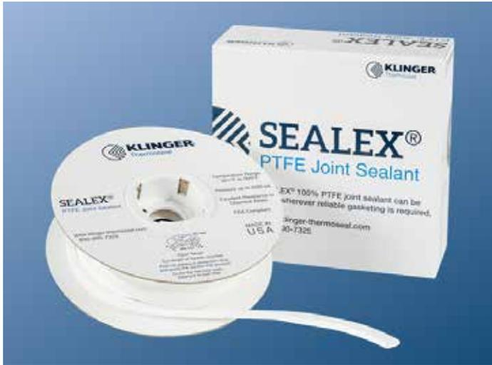
Sealex® joint sealant, specially processed, pure, expanded PTFE on a roll, provides soft, highly compressible gasketing for longer life and trouble-free sealing. Its form-in-place versatility also cuts maintenance and storage costs. The high compressibility of Sealex® enables it to effectively fill flange imperfections for a tight, leak-free seal. Under pressure, it provides a wide, thin, ribbon-like seal.
