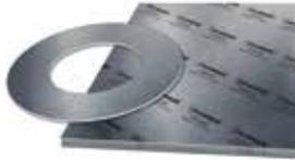
Graphite gasket material with a stainless steel tang insert. KLINGER® Graphite Laminate PSM has a 0.1 mm thick perforated stainless steel insert. The insert aids material handling properties and also increases the blow-out resistance. The insert is mechanically bonded to pure exfoliated graphite and therefore does not rely on adhesive. KLINGER® Graphite Laminate PSM is suitable for hot water.
