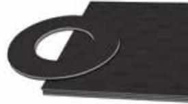
A universal high-pressure gasket material with a low carbon steel woven mesh insert that improves stress relaxation and makes this material suitable for fluctuating temperatures and pressures. C-4408 has good resistance to oils, fuels and hydrocarbons, and is manufactured with aramid fiber reinforced with a nitrile binder.
