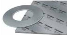
The pure graphite gasket sheet with a smooth stainless steel insert. SLS is suitable for universal use especially in combination with weak flanges at high temperatures and for sealing of liquid level gauges. The gasket material consists of pure exfoliated layers of graphite, which are mechanically bonded to a 0.05 mm thick, smooth, stainless steel insert. The insert aids material handling properties and also increases blow-out resistance.
