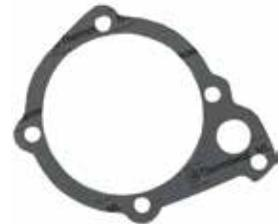
ML-S723 is a controlled-swell gasket material intended for heavy-duty applications. ML-S723's blended styrene-butadiene and natural rubber binder provides exceptional sealability and conformability with low creep relaxation. Thickness increase, in the presence of oils and fuels, aids the sealing of irregular flange surfaces. Typical applications include diesel engine oil pan gaskets and gear plate and rear seal carrier gaskets with intermittent operating temperatures up to 350°F (177°C).
