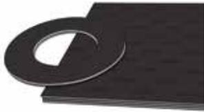
A high-pressure gasket material. The expanded metal reinforcement is a galvanized low carbon steel insert which increases the compressive strength and pressure capability. Has higher resistance against blowouts. C-4509 is manufactured with carbon fibers and special high-temperature resistance additives and reinforced with a nitrile binder.
