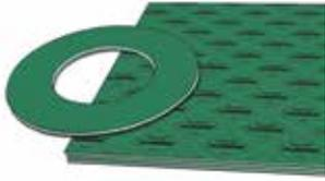
A universal gasket material with outstanding stress relaxation and resistance to hot water and steam making it suitable for a wide range of applications. C-4430 is manufactured with a combination of aramid fiber and fiberglass reinforced with a nitrile binder.
