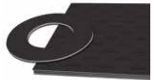
This gasket material is a good steam sheet with good anti-stick properties. Use this material in process industries. C-6400 is manufactured with synthetic fiber reinforced with an SBR binder.
