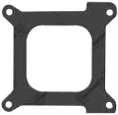
ML-5270 is a synthetic fiber and polychloroprene binder material that is resistant to refrigerants and oil mixtures. Typical applications include gaskets in hermetic and semi-hermetic compressors and oil pan gaskets in heavy-duty diesel engines with intermittent operating temperatures up to 350°F (177°C).
