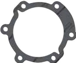
RG-N120 is a reinforced cellulose gasket material with a nitrile butadiene rubber binder and inorganic fillers that provides very good crush resistance at high flange pressures. RG-N120 seals oils, water, and coolants in applications such as small engine intake and cover gaskets, automotive water pump and throttle body gaskets. RG-N120 is suitable for applications with intermittent operating temperatures up to 350°F (177°C).
