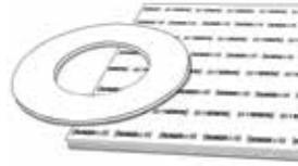
Superior performance sealing in critical applications. KLINGER®tc-1006 is a high quality, yet cost-effective biaxial oriented modified PTFE gasket material with barium sulphate that offers superior sealability, excellent torque retention, and reduced creep relaxation. Use gaskets from KLINGER®tc-1006 for most chemical applications. This gasket material is free of pigments and meets FDA conformity.
