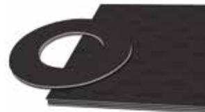
This gasket material is a good choice for liquids and steams with low-temperature and low-pressure applications. Controlled swelling in oils and fuels provides very good adaptability to any sealing surface. Offers excellent conformity to flanges at low surface bolts. C-6327 is manufactured with synthetic fiber reinforced with a modified SBR binder.
