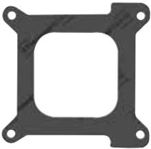
RG-N100 is a nitrile butadiene rubber, reinforced cellulose fiber and mineral filler general purpose gasket material. Its low density provides good conformability in sealing fuels, oils, and water in applications such as automobile water pumps, miscellaneous cover gaskets, and many small engine applications. RG-N100 is suitable for applications with intermittent operating temperatures up to 350°F (177°C).
