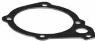
ML-N102 is a synthetic fiber and nitrile butadiene binder gasket material with good resistance to refrigerants and lubricating oils. Typical applications include heavy-duty diesel engines and compressors with intermittent operating temperatures up to 450°F (232°C).
