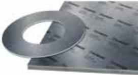
Graphite laminate sheet without reinforcement. HL is a homogeneous sheet made from flexible graphite foil layers. It is the standard industrial grade graphite sheeting with superior chemical resistance. The flexible graphite material is highly compressible and compactable allowing for low gas permeability with low electrical resistance. The grade is especially superior working with enamel surface as well as against strongly corrosive media.
