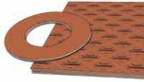
An excellent high-performance material. The expanded metal reinforcement is a galvanized low carbon steel insert which makes this material suitable when vibrations are present. C-4439 is manufactured with a combination of fiberglass and aramid and inorganic fibers reinforced with a nitrile binder.
