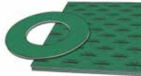
A universal gasket material for use in a wide range of applications and is a good general-purpose material. C-4324 is manufactured with a combination of synthetic high-performance fibers reinforced with a nitrile binder.
