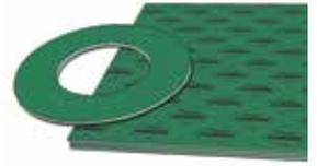
Has an expanded metal reinforcement. The galvanized low carbon steel insert makes this material suitable for conditions with high thermal and mechanical stress. C-4409 is manufactured with synthetic fiber reinforced with a nitrile binder.
