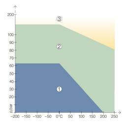
In area ① the gasket material is suitable using common installation practices subject to chemical compatibility.
