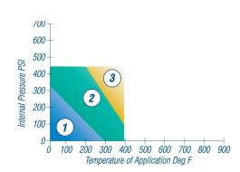
In area 1 the gasket material is suitable using common installation practices subject to chemical compatibility.
