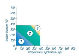
In area ① the gasket material is suitable using common installation practices subject to chemical compatibility.
